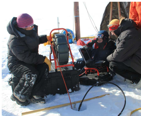
Glaciologist Lora Koenig [left] operates a video recorder that has been lowered into the bore hole to observe the ice structure of the aquifer in April 2013. Image credit: University of Utah/Clément Miège
