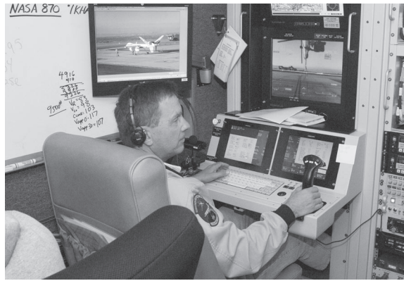
NASA research pilot Mark Pestana flies the Ikhana unmanned aircraft remotely from the ground control station at NASA Dryden. Credit: Tom Tschida.
