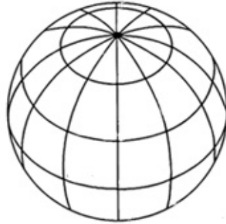
Figure 3. Convergence of longitude lines produces shrinking of 1^\circ \times 1^\circ grid cells toward the poles.
