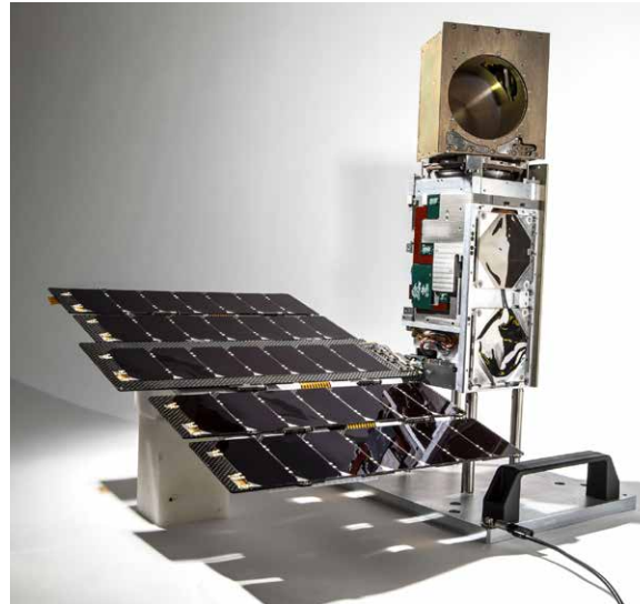
Figure. The TROPICS Pathfinder satellite, pictured above, was launched on June 30, 2021. The satellite body measures approximately 10 cm x 10 cm x 36 cm (-4 in x 4 in x 14 in) and is identical to the six additional satellites that will be launched into the constellation in 2022. The golden cube at the top is the microwave radiometer, which measures the precipitation, temperature, and humidity inside tropical storms. Image credit: Blue Canyon Technologies
