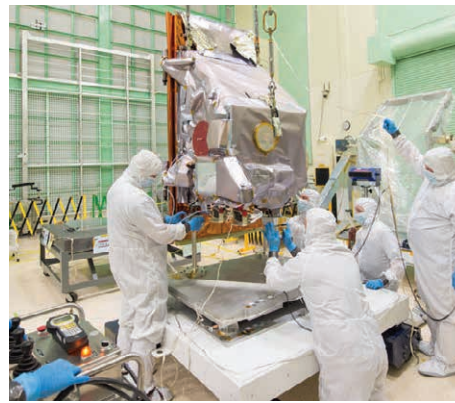
Figure 4. [Left] Engineers at GSFC work on TIRS-2, which will measure temperatures on Earth's surface from the Landsat 9 satellite. [Right] Diagram of TIRS-2 showing main components. Description available at go.nasa.gov/3A1nmk7 . Photo credit: NASA
