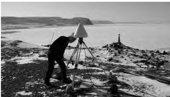
Earl Frederick calibrating the Operation Ice Bridge ground GPS antenna. Credit: Jim Yungel.
