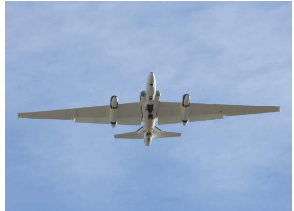
During the Integrated Precipitation and Hydrology Experiment, NASA's high-altitude ER-2 aircraft carries three radars and a radiometer to measure rainfall from 65,000 ft (~20 km). Image credit: Tony Landis [NASA's Armstrong Flight Research Center]
