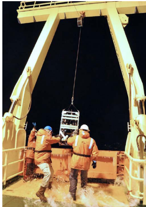
Water intrusion during recovery of the inherent optical properties (IOP) package. The IOP package is an assemblage of instruments that collect data for temperature, salinity, depth, and light absorption due to particulate and dissolved components. Image credit: NASA
