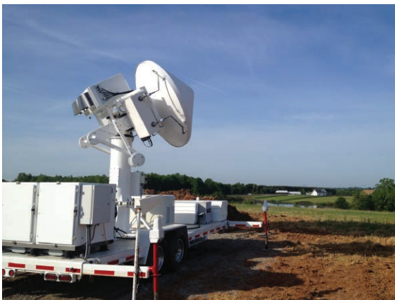
Set up on a ranch in Rutherford County, NC, NASA's Dual-frequency, Dual-polarization, Doppler Radar (D3R) is one of several ground radars measuring rain as it falls from clouds. It has the same two frequencies as are on the GPM Core Observatory satellite. Image credit: David Wolff [NASA's Wallops Flight Facility]
