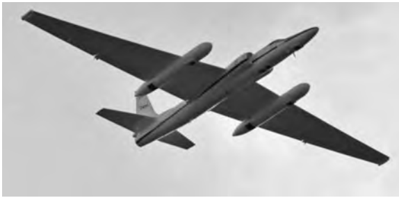
Figure 5. [left] NASA's Earth Resources-2 (ER-2) aircraft carries the AVIRIS sensor. Figure 6. [right] NASA's Gulfstream G-III aircraft has the UAVSAR mounted underneath. Image credit: NASA
