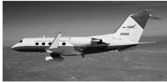
Figure 5. [left] NASA's Earth Resources-2 (ER-2) aircraft carries the AVIRIS sensor. Figure 6. [right] NASA's Gulfstream G-III aircraft has the UAVSAR mounted underneath. Image credit: NASA
