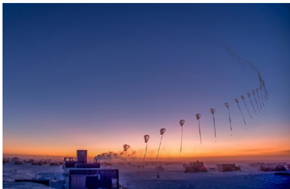
This time-lapse photo from September 10, 2018, shows the flight path of an ozonesonde as it rises into the atmosphere over the South Pole from the Amundsen-Scott South Pole Station. Scientists release these balloon-borne sensors to measure the thickness of the protective ozone layer high in the atmosphere. Image credit: Robert Schwarz/University of Minnesota
