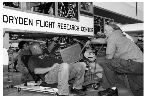
HIWRAP is a new, advanced radar instrument that will allow NASA scientists to measure surface winds above the ocean inside a hurricane. Lihua Li [ left ], Goddard Space Flight Center engineer, Steve Crowell [ sitting ], Northrop Grumman mechanic; and Ken Wilson [ kneeling ], NASA's Global Hawk crew chief, worked earlier this week to integrate the HIWRAP instrument onto NASA's Global Hawk . HIWRAP is one of 14 instruments that will be deployed on three NASA aircraft during GRIP. Image credit: NASA's Dryden Flight Research Center
