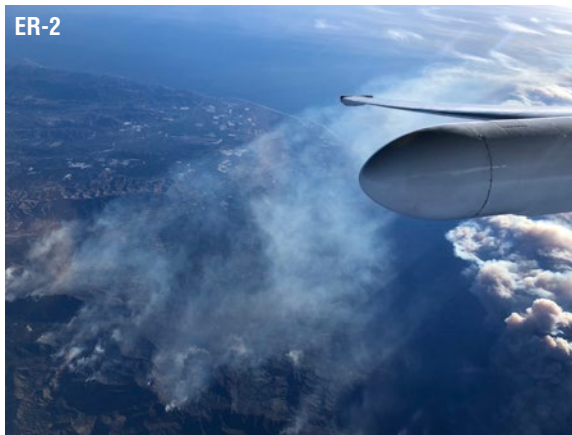
Figure 1. The top photo shows the NASA ER-2 on takeoff. This civilian version of the U-2 spy plane is capable of flying at altitudes greater than 70,000 ft (~21 km) making it an invaluable platform for simulating satellite measurements. The lower image shows the ER-2 in flight during FIREX-AQ, taking measurements high above a smoke plume in California. Photo credits: NASA
