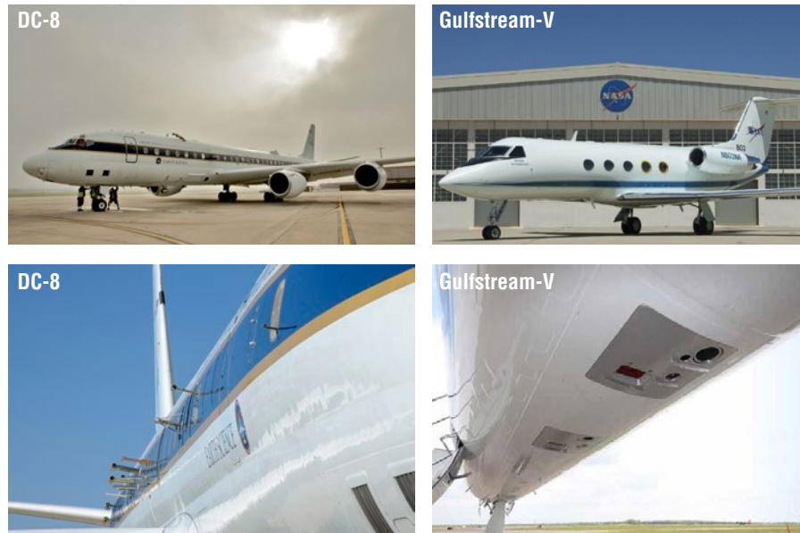
Figure 2. Shown here are two ASP aircraft that have been custom designed to accommodate remote sensing and in situ instruments for making Earth observations. The top left photo shows ASP's DC-8. This is NASA's "workhorse" aircraft—both because it can carry heavy payloads and because it is frequently called upon for service. The lower left photo shows the windows on the DC-8 that were modified to accommodate air sampling probes that take in situ trace gas and aerosol measurements. The top right image shows the NASA Gulfstream-V (G-V) aircraft. The lower right photo shows the underbelly of the G-V that has been modified to accommodate a waveform scanning lidar to measure sea surface altimetry. This configuration of the G-V was used for Surface Water and Ocean Topography (SWOT) cal/val activities. More details about these two aircraft appear in Table 1 on page 8. Photo credits: NASA
