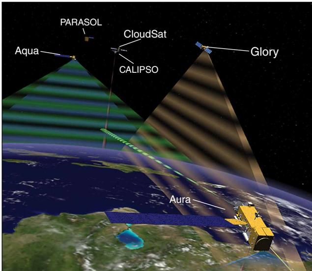
The close proximity of the different spacecraft within the A-Train allows for near-coincident observations between instruments on different spacecraft, providing scientists additional capabilities in their pursuit of answers about the Earth and its climate. Credit: NASA
