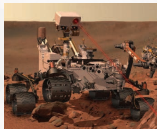
This artist's concept depicts Curiosity as it uses its Chemistry and Camera (ChemCam) instrument to investigate Mars. Image Credit: NASA/Jet Propulsion Laboratory-Caltech
