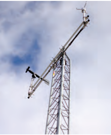
Land-based weather monitoring station, Holland, Michigan
