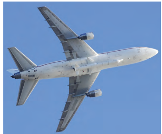
Pegasus XL expendable rocket affixed to the bottom of the L-1011 Stargazer . Image credit: NASA
