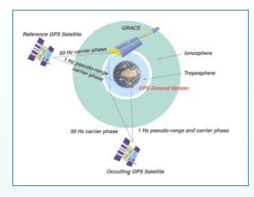
This diagram, originally provided by GFZ, illustrates how the occultation process works. The GRACE satellite tracks a GPS satellite as it "rises" and "sets" through the limb of the atmosphere, while a second GPS serves as a reference point.
