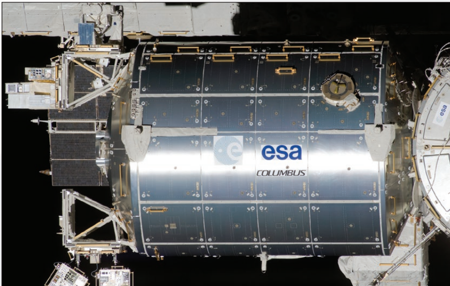
[Above] The ISS-RapidScat payload will be berthed to the Columbus module onboard the station—a seven-meter-long research laboratory installed in February 2008.
