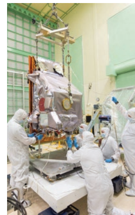
Engineers at NASA Goddard work on TIRS-2, which will measure surface temperatures on Earth's surface from the Landsat 9 satellite. Photo credit: NASA
