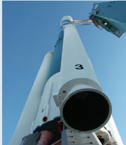
This image provides a view of the Delta II 7320-10C launch vehicle looking into the nozzle end of one of the three Graphite Epoxy Motors that serve to double the thrust of the rocket to more than 500,000 pounds per force (thrust). Image credit: Steve Greenberg
