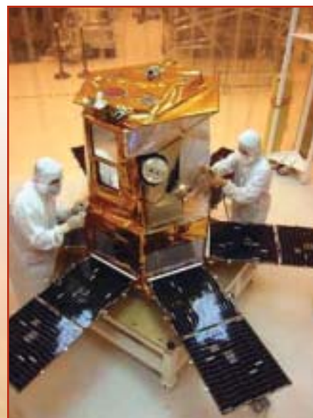
The SORCE spacecraft with the Solar Arrays deployed at Orbital Sciences Corporation, during Integration and Test (I&T).
