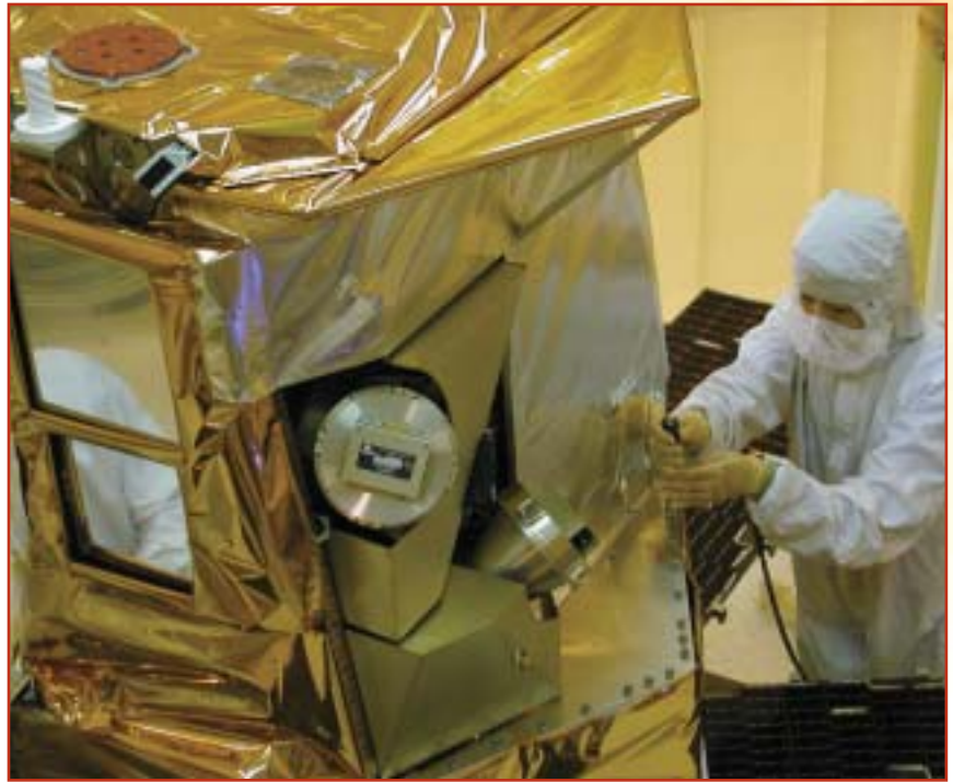
A SORCE engineer is checking the bolts connecting the IM platform to the spacecraft bus.
