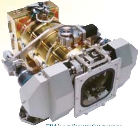
TIM is a radiometer that measures TSI with 0.01% absolute accuracy.
