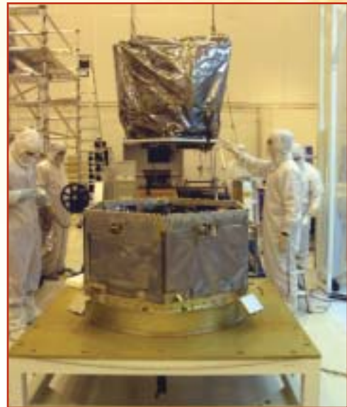
After delivery to the Orbital Space Systems Group in Dulles, Virginia, the Instrument Module (IM) is mated to the spacecraft bus.
