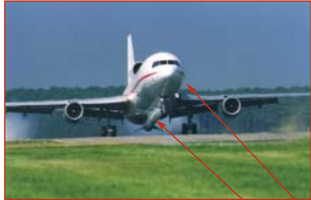
Takeoff of the Pegasus XL space launch vehicle and its L-1011 carrier aircraft.
