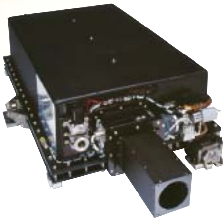
Two identical and fully redundant SOLSTICE instruments measure ultraviolet (115 to 320 nm) solar and stellar radiation.
